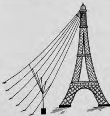
Fig. 1. Schematic Arrangement of the Actual Antenna Supported by the Famous Eiffel Tower.
